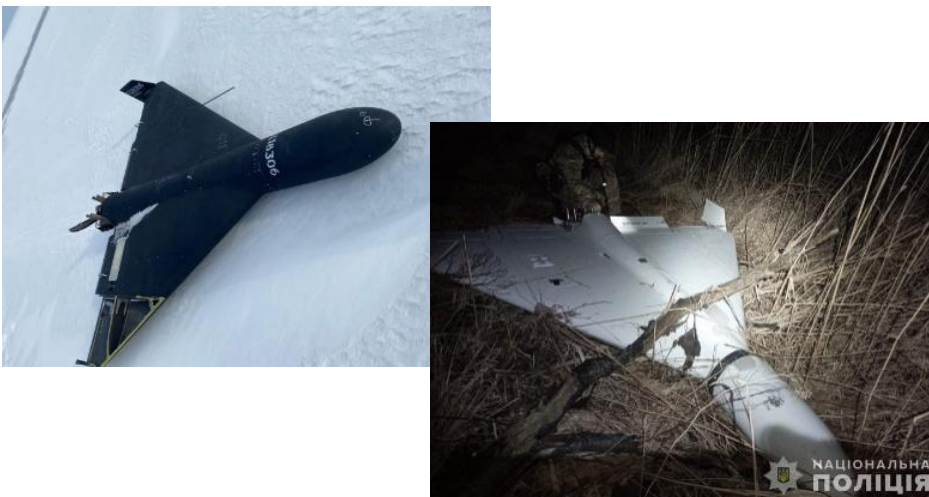
Figure 1 -- Shahed attack UAVs suppressed by electronic warfare systems without signs of kinetic impact.
